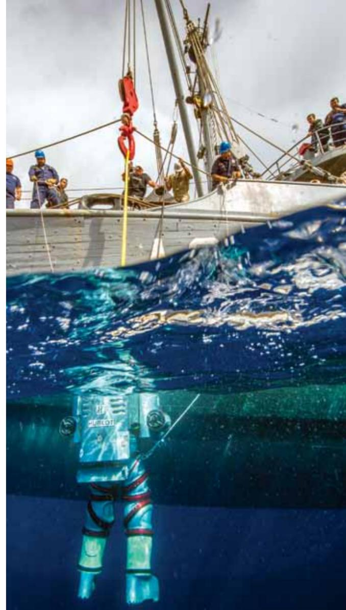
The one atmosphere Exosuit allows hours of dive time with zero decompression time
